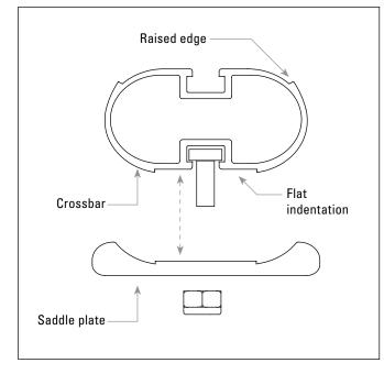
3. Now insert the bolts through the holes in the saddle plates. Center the crossbar between the left and right corner units by adjusting the amount of crossbar that protrudes from each end of saddle plate.
