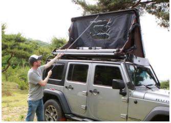
4. Tuck the excess material into the Skycamp on the front, back and side:
