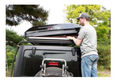
5. Pull down on the hard shell, and securely fasten the locks (or straps). Make sure the strap is tight by adjusting (twisting) the bottom U-shaped piece.
