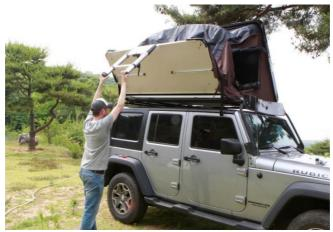
3. Reach into the Skycamp to grab the black nylon strap attached to the top of the shell. Pull down on the strap to close the hard shell:
