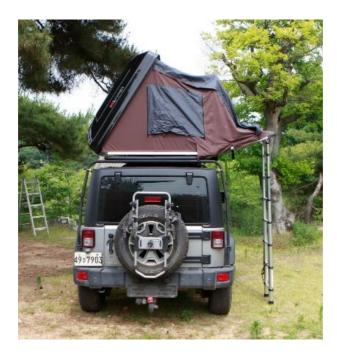
The ladder should NOT be over-extended as it does not offer enough support, and is should not be too vertical either.
